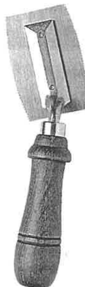
Fig. 19-7—A veneer saw is made specifically for cutting veneer.
