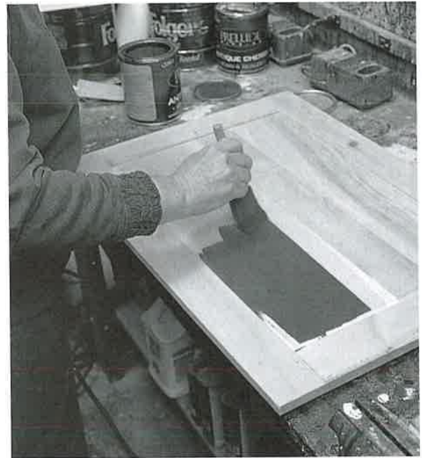
Fig. 33-2 — If painting over bare wood, a primer is always needed to seal the wood.
